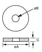
Note: Snubbing washers are not supplied by Mackay Consolidated Industries. The Standard material should be low-carbon steel
